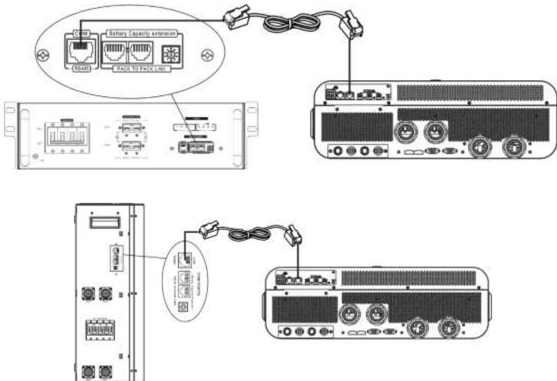
\* For multiple battery connection, please check battery manual for the details.
