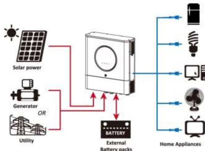
**Figure 1 Basic hybrid PV System Overview**
