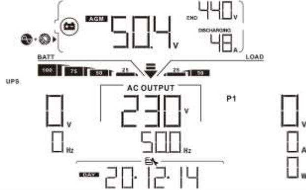
Load in VA=2.4kVA, Output frequency=50Hz
