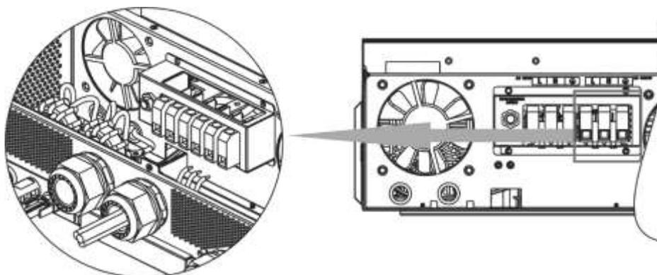
6. Make sure the wires are securely connected.
